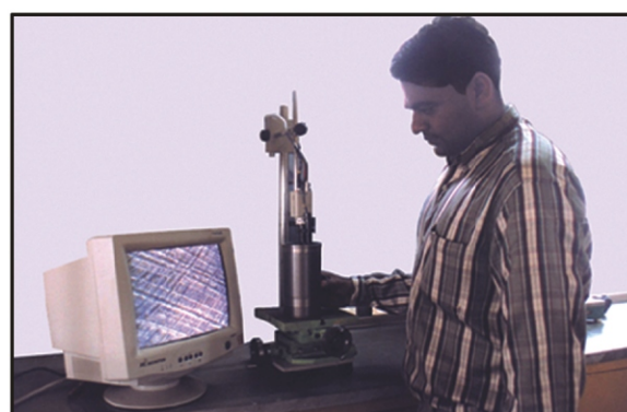
Special Purpose Microscope Type VW SPM 4 (Cylinder Liner Surface Honing Texture Viewing & Photographing)
